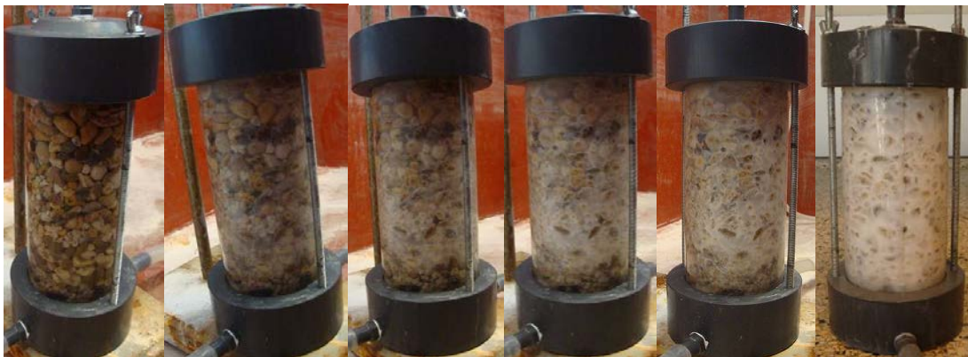
Figure 32: Gravel packed column IV (beginning, 30min, 60min, 100min, 240min later and end)
