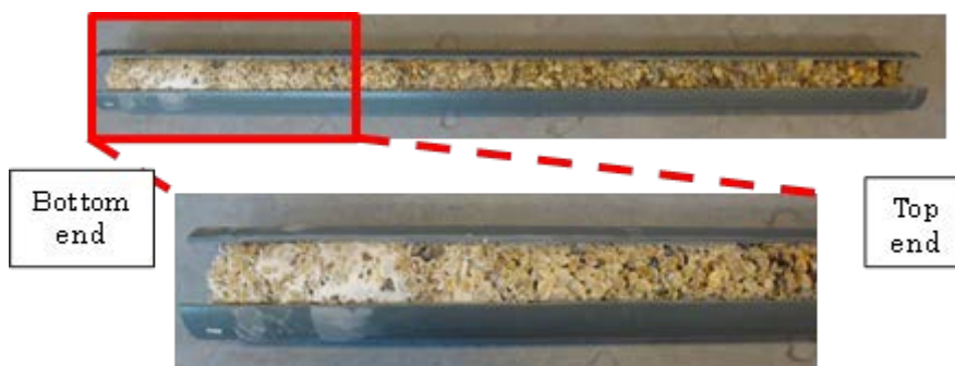
Figure 34: Cemented sample after removed from column
