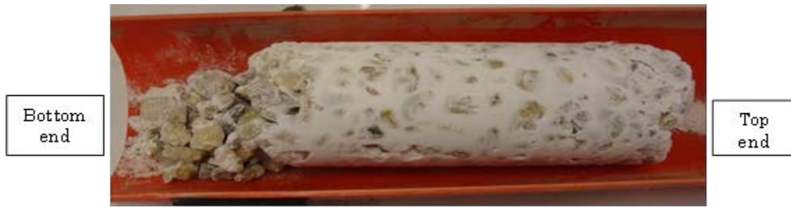
Figure 33: Gravel treated with cementation (column W)
